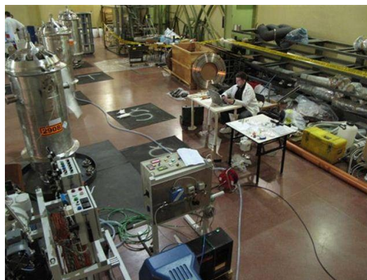
FIG. 15. Drying and vacuuming of TUK-19 casks.
