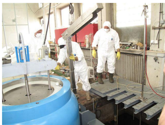
FIG. 13. Loading a basket into SKODA cask.
