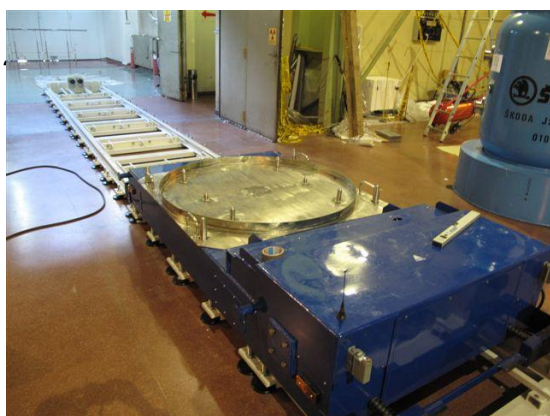
FIG. 9. Cask rail-transfer system.
